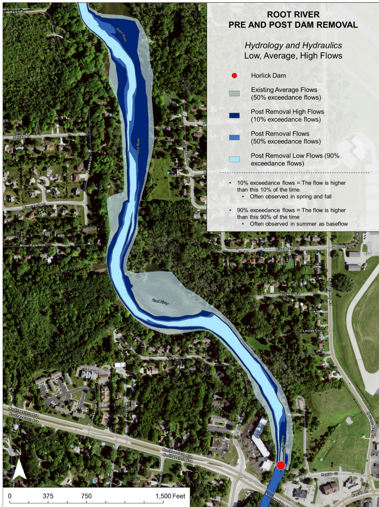
Figure 24: Post dam removal exceedance flows (10%, 50%, 90%) for the Root River reach
