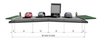
The preferred alternative is a four lane undivided roadway with 12' inside and 14' outside lanes. Bicycle accommodations are provided on the widened outside lane. Turn lanes will be provided at Circle Drive and Rivershore Drive. The intersection of CTH MM with STH 38 will be reconstructed and realigned as part of the project.
